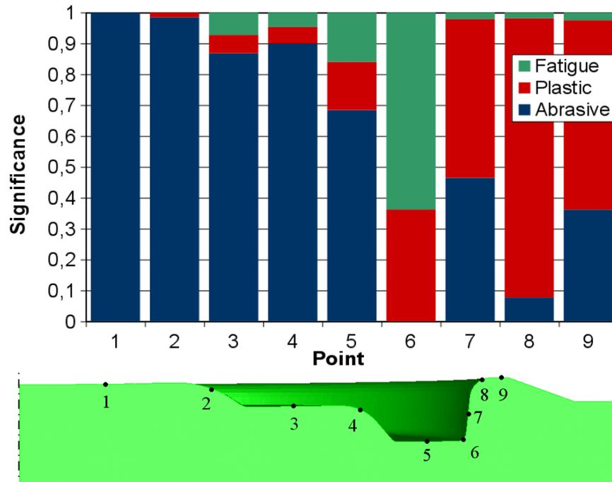
**Figure 3:** Wear significance values and measurement points at a lower die
