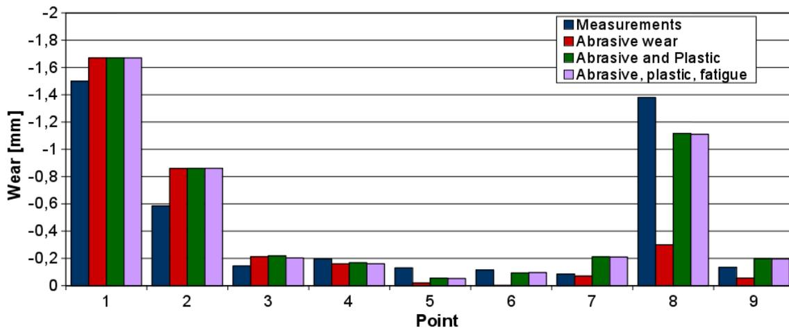
Figure 4: Total wear values of different models compared to measurements in lower die.
