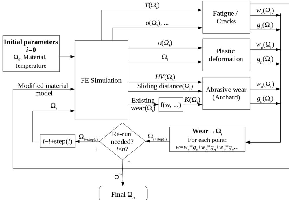
Figure 1: Block diagram of proposed hybrid model
